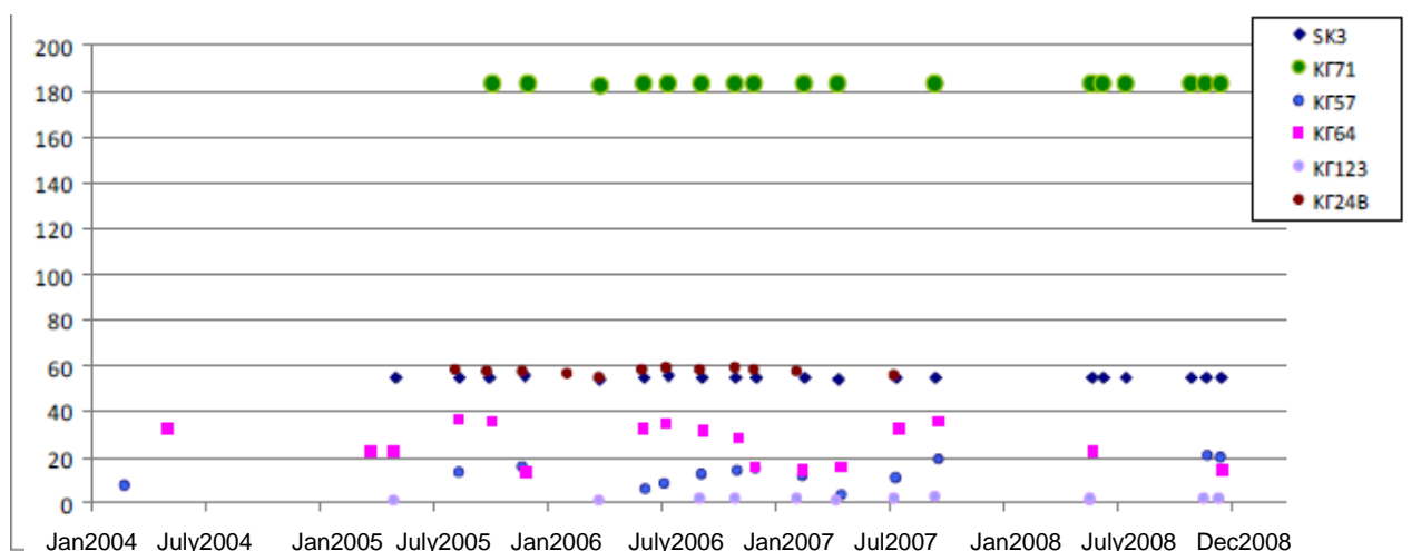
Figure 4.26: Variations of the groundwater level of drillings in GR0500010 (RBMP of Epirus, Del.10)
